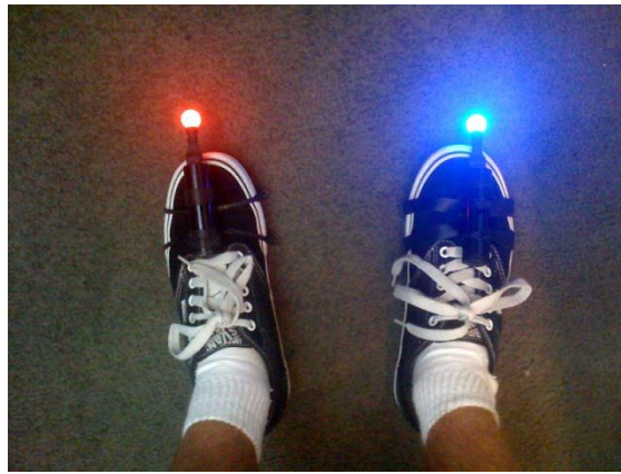
Figure 4. LED devices attached to right and left shoes of the user (tracked by web cameras).
