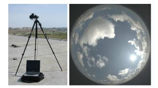
Figure 1: The camera with  $180^{\circ}$  fisheye lens and laptop on the roof of our building (left). This is a typical assembled probe (right) taken with the fisheye lens and neutral density filter spanning the 17 stops of the sky and sun.
