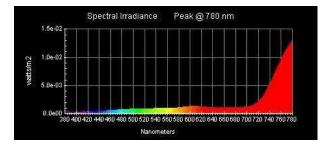
Figure 5: The spectral calibration of the 3.0 ND Kodak WRATTEN Filter, showing a gentle increase in the visible range from blue to red. A significant amount of IR light is transmitted.
