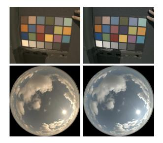
Figure 4: The neutral density filter while reducing the amount of light introduces a chromatic change as well. To correct for this a color chart was photographed with and without the ND filter. These images were then used to solve for a color correction matrix.
