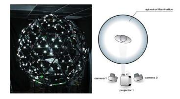
Figure 2: Acquisition setup for ICT-3DRFE. Left: LED sphere with 156 white LED lights. Right: Layout showing the positioning of the stereo pair of cameras and projector for face scanning.
