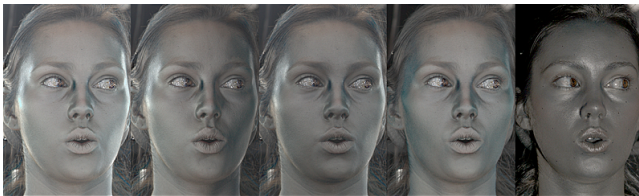
Figure 3: Emily’s specular component under the four gradient lighting conditions (all, left, top, front) and single frontal flash condition, obtained by subtracting the cross-polarized images from the parallel-polarized images.
