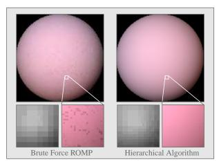
**Figure 2:** Spatial coherency of brute-force compressive light transport sensing (left) versus hierarchical compressive light transport sensing (right). The reflectance functions (128×128) are in both cases reconstructed from 1000 measurements using 100 Haar wavelet coefficients. For each algorithm, a detail is shown to better illustrate the differences in coherency. Additionally, a single reflectance function from this detail is shown on the bottom left of each example.
