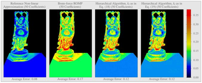
**Figure 7:** *Error Comparison.* False color images of the relative error with respect to a reference reflectance field. From left to right: an error image showing a baseline 50 coefficient non-linear Haar wavelet approximation, the error on brute-force ROMP, the error on the presented hierarchical algorithm, and the error on the hierarchical algorithm using the alternative formulas (19) for the per-level sparseness and difference sparseness.
