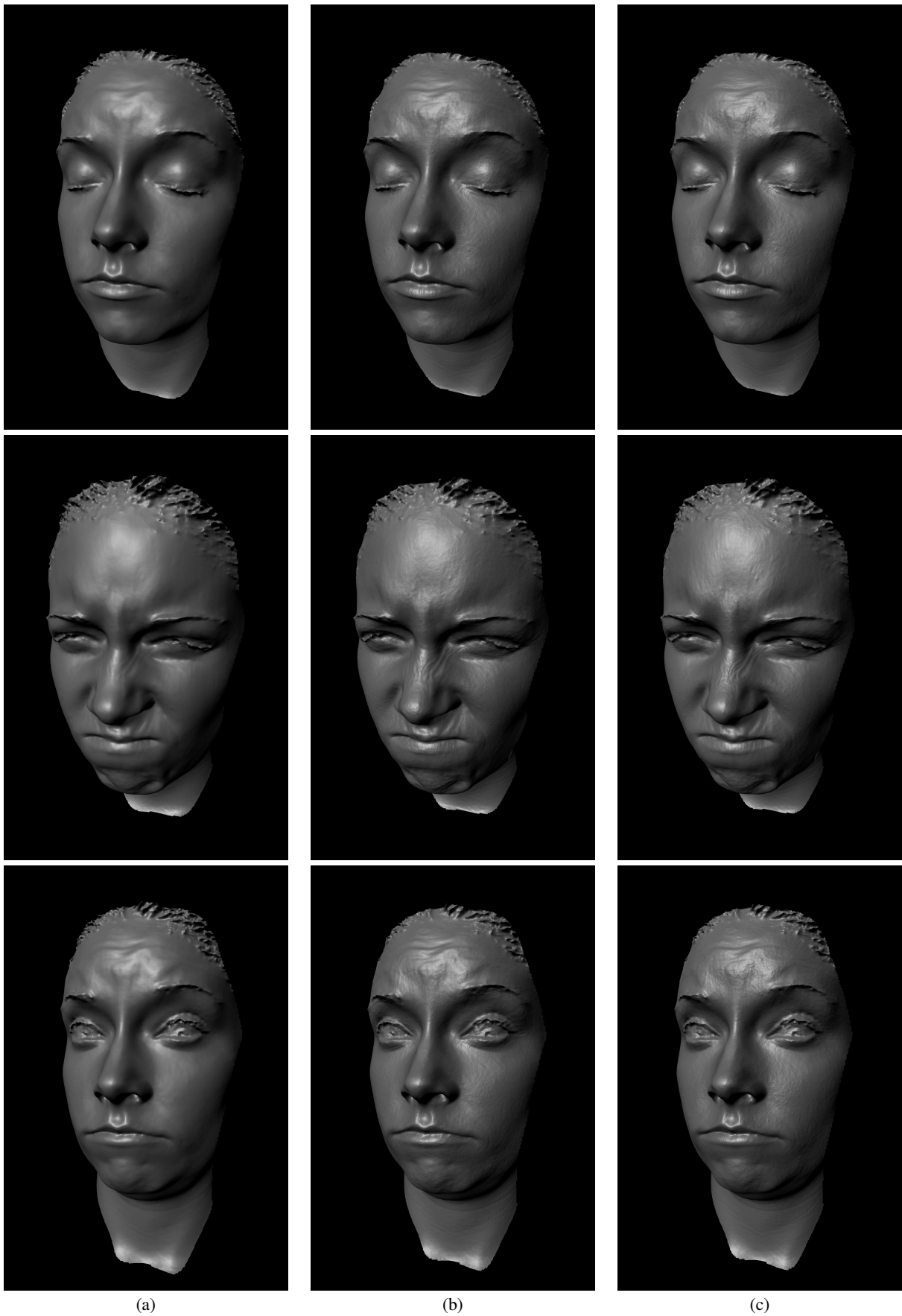
Figure 3: (a) Base geometry. (b) Geometry optimized with synthesized specular normal map. (c) Geometry optimized with captured specular normal map. This figure shows the geometry optimization results of the same person with different expressions.
