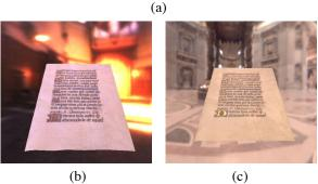
Figure 7. Linear Light Source Reflectometry. The spatially-varying surface reflectance parameters of an illuminated manuscript are recorded using a simple apparatus based on a translating linear light source. The per-pixel estimates of diffuse and specular parameters, as well as surface normals, can be used to create photoreal real-time renderings (below) of the artifact from any viewing angle and in any lighting environment.
