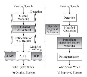
Figure 1: Comparison of two speaker diarization systems. (a) Original system introduced in [7]. (b) Proposed, improved system in this paper. Notable features in each system are highlighted. LFC: leader-follower clustering, SAD: speech activity detection, SCD: speaker change detection, AHSC: agglomerative hierarchical speaker clustering, iGMM: incremental Gaussian mixture model, and ICR: information change rate.
