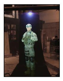
Figure 3: Interactive character projection onto a transparent screen creates the illusion of a hologram.
