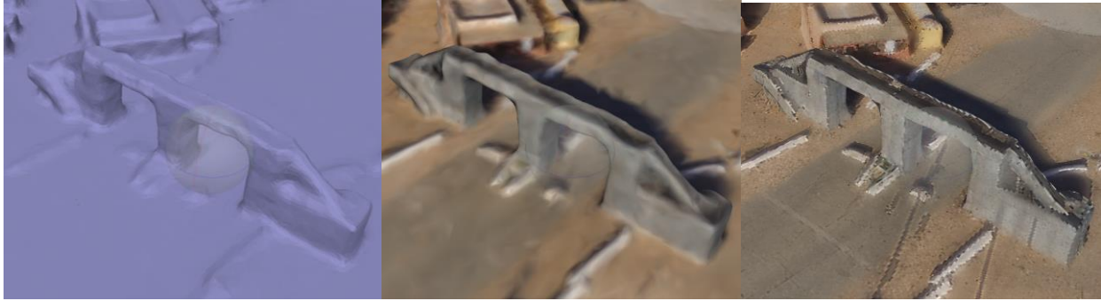
Figure 7. Mesh reconstruction and texturing steps. From left to right: flat-shaded mesh; mesh with per-vertex color data; mesh with texture applied. Images generated with Agisoft PhotoScan.
