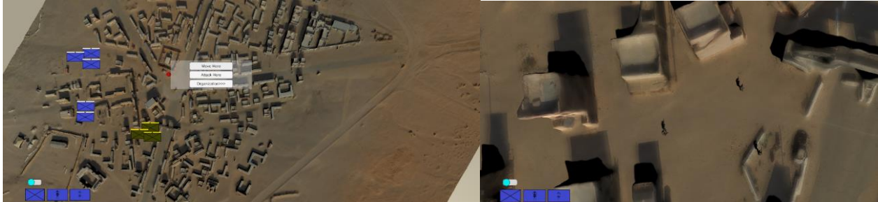
Figure 11. Prototype mission planning/rehearsal in the Unity3D Game Engine, using a city acquired through the pipeline. Left: A wide view of a simulated city showing aggregated icons. Note the menu for placing units (lower left of image) and the context menu for the selected unit (center). Right: A closer view of the same scene, showing individual Soldier entities.
