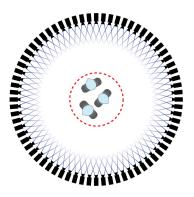
Figure 2. Surrounding viewers with a dense array of picoprojectors. Placing the projectors sufficiently far from the viewers (with correspondingly longer lenses) permits an arbitrary numbers of projectors to be used, achieving any desired scene resolution.
