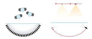
Figure 3. (Left) Top down view showing an array of picoprojectors behind a vertically diffusing screen, achieving a horizontal-parallax-only display. (Right) We simulate such an array by flashing different views of the scene along the arc from a single pico-projector. The camera records the summed effect of these flashes using long exposures.
