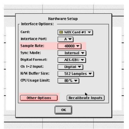
3. For each Interface Port(A and B) on each MIX Card (#1 and #2) hit the "Other Option" button This will bring up a dialog to control the input source of an 888. Set all channels to use their digital inputs
