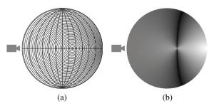
Figure 4: (a) Hemispherical angular map representation of directions of linear polarization for independently observing the specular and subsurface reflection for a full sphere of illumination. The full sphere is derived by mirroring this hemisphere. The camera is assumed to lie to the left. (b) Attenuation of specular reflection, represented in the same space as (a). Near the Brewster angle the reflection is weak, making recovery of true specular reflectance unstable.
