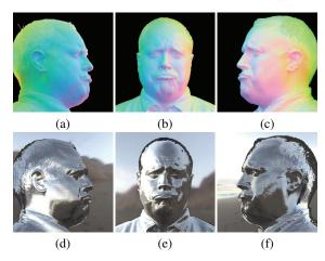
Figure 6: Normal map capture of live performances. (a,b,c) Surface normal maps from three viewpoints derived from the same set of four gradient illumination conditions of a live performance. (d,e,f) Environment mapped renderings using the maps to show normal detail.
