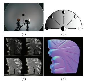
Figure 9: Acquiring normals for a highly specular surface. (a) Reflective hemisphere to create continuous gradient illumination, showing the viewing aperture, subject, and half-covered light bulb. (b) Diagram of a half-covered light bulb producing gradient illumination. (c) Left, top, front, and full gradient illumination conditions on a polished obsidian sculpture. (d) Computed normal map from the specular reflection.
