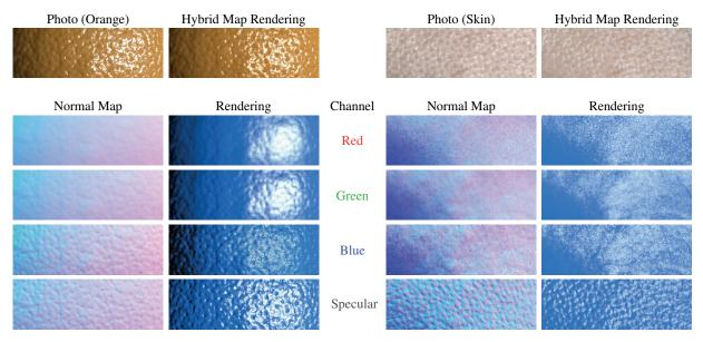
Figure 8: Normal map comparison for specular and diffuse color channels of an orange and human skin. In both cases, shorter-wavelength illumination yields more surface normal detail. The blue channel of the orange is extremely dark leading to noisy blue normals. In both cases, the specular channel contains the most surface detail.
