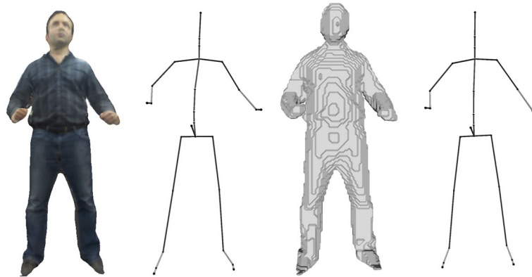
Figure 7. The voxelization produces the skeleton similar to the one extracted from original mesh. Left: original mesh and its skeleton. Right: voxel representation of original mesh and its corresponding skeleton.
