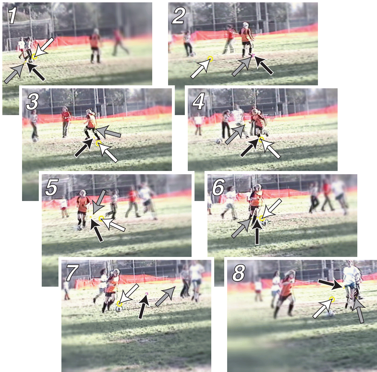
Figure 5. Demonstration of the system in operation on an outdoors video clip ( 640 \times 480 at 30 frames/s, analog interlaced source) processed in a fully automatic manner. Grey arrows indicate current position of covert attention, black arrows current eye position, and white arrows current head position. (1) In this first frame, covert attention, eyes and head are focused onto the soccer ball. (2) The player at the center of the image (orange shirt) starts running towards the ball and becomes highly salient; this has elicited an eye saccade that is just reaching completion in this frame. The head is also moving towards this player, but more slowly so that it lags somewhat behind. (3) Attention, eyes and head are now focused onto that central player and smoothly pursue her. (4) A new player (white shirt) very rapidly enters the field of view and has attracted covert attention, but not in a sufficiently reliable manner to elicit a saccade. (5) Attention, eyes and head smoothly track (with some small lag) the central player (orange shirt), who now has the ball. (6) That player makes a sharp turn and prepares to kick the ball. (7) The player with the white shirt also makes a sharp turn, and is reliably attended to, yielding a saccade, here caught with the eyes in mid-flight between old (close to head) and new (close to covert attention) positions. (8) Attention, eyes and head regroup close to the player with the white shirt, who is preparing to intercept the ball. No parameter tuning was used to process this or other clips. The visual input is very noisy, low-quality, richly textured and cluttered, and the camera moves substantially, creating large full-field motion transients and changes in object appearances.
