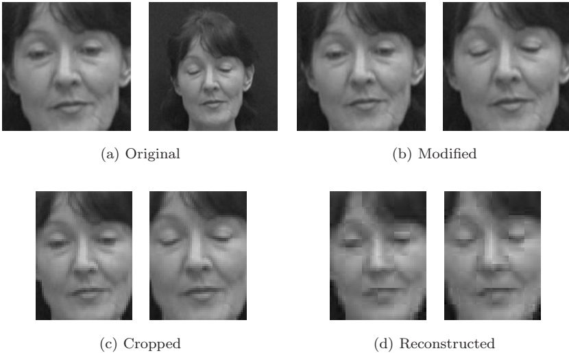
Fig. 1. Two consecutive frame images after face detection. (a) By the original face detection algorithm ( 32 \times 32 pixels). (b) By the modified version considering the face size of the previous image frame ( 32 \times 32 pixels). (c) By the more refined version considering the cropped faces with a general ratio of width and height ( 24 \times 32 pixels). (d) By the reconstructed procedures from the face features ( 24 \times 32 pixels). Note that we have zoomed all the images by 2\times for better display.
