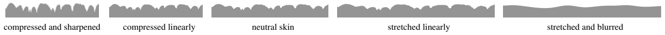
Figure 4: Stretching and compressing a measured OCT skin profile, with and without convolution filters to maintain surface length.
