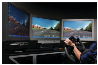
Figure 1. This picture shows the 3-screen visual display utilized in this study
