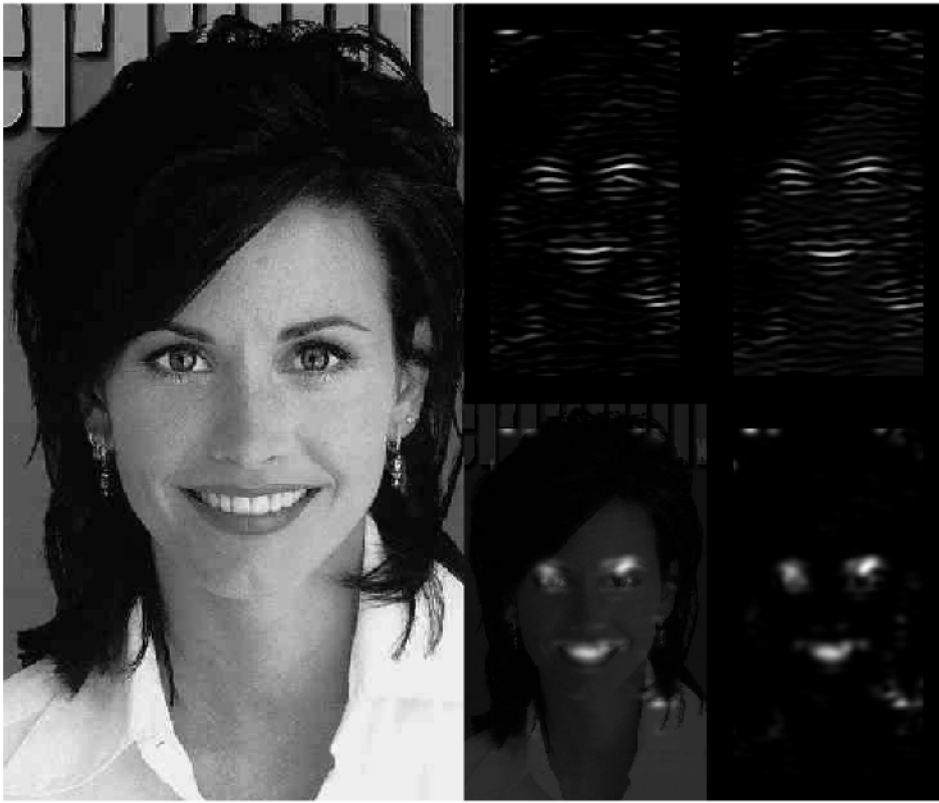
Figure 4. Illustration of facial feature detection by the quadrature demodulator network shown in Figure 3. Left , Input image. Right (clockwise from top left), the real part of the result of convolution with a 2D Gabor wavelet; the imaginary part from the same convolution (both of these representing the phase-sensitive simple-cell responses); the squared modulus A^2(x, y) , representing complex cell response; and this result superimposed on the original (faint) image, illustrating feature detection and localization.
