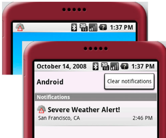
Figure 4.5 The Notification -based alert the WeatherAlertService displays to the user when severe weather is detected in the forecast
