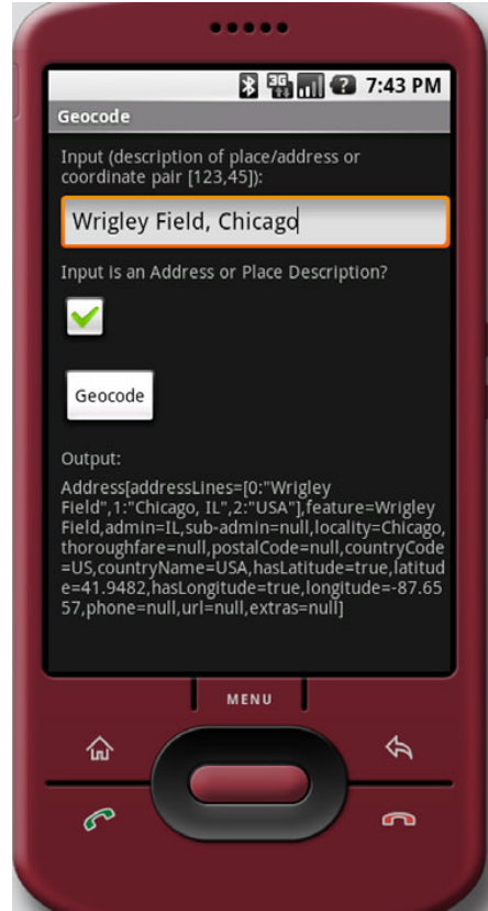
Figure 11.8 A Geocoder usage example that demonstrates turning an Address String into an Address object that provides latitude and longitude coordinates
