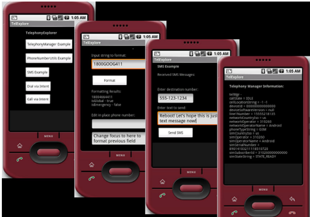
Figure 7.1 TelephonyExplorer main screen, showing all the related activities the sample application performs
