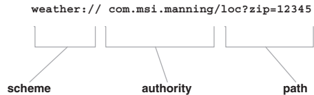
Figure 4.2 The portions of a URI that are used in Android, showing scheme, authority, and path
