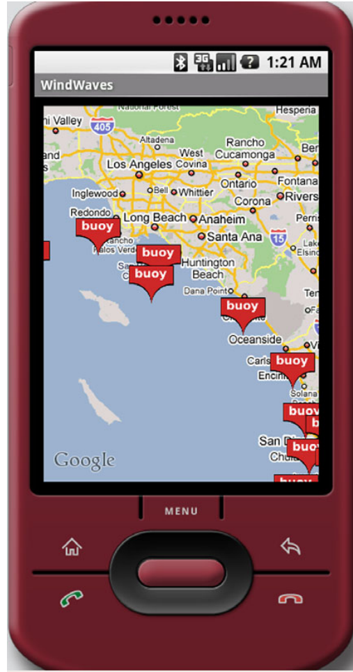
Figure 11.6 The MapViewActivity from the Wind and Waves application showing a MapActivity with MapView
