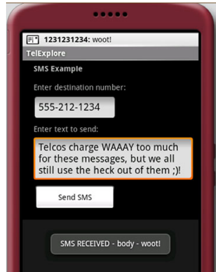
Figure 7.4 An Activity that sends SMS messages and an example of an alert based on a received SMS message
