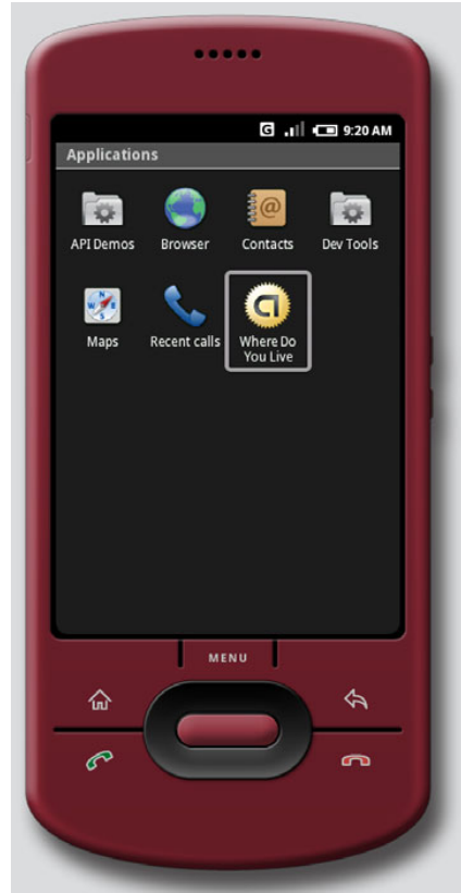
Figure 1.7 Applications are listed in the launcher based on their IntentFilter . In this example, the application “Where Do You Live” is available in the LAUNCHER category.
