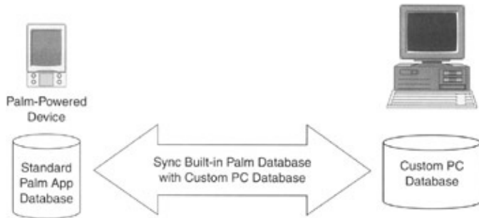
Figure A.2: Synchronization between the custom PC database and the standard PDA application database.
