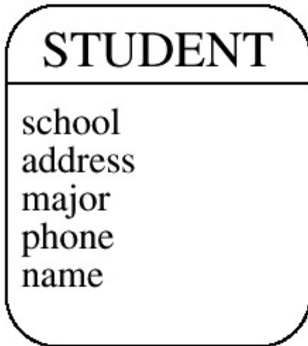
Figure 10.1: Barker/Oracle-Like Notation: An ER Diagram with One Entity and Five Attributes
