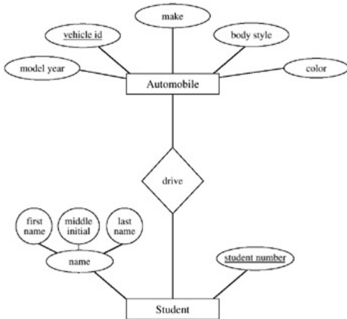
Figure 3.5: An ER Diagram of the STUDENT–AUTOMOBILE Database
