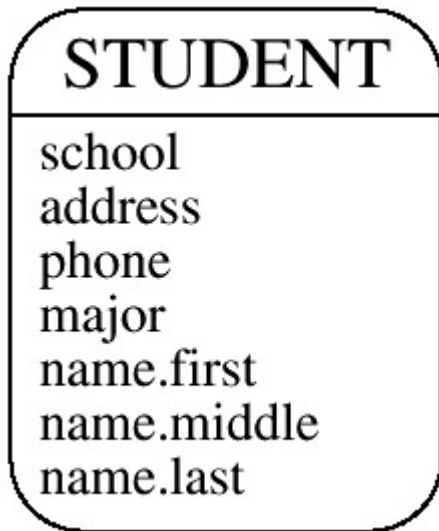
Figure 10.2: Barker/Oracle-Like Notation: An ER Diagram with a Composite Attribute — name
