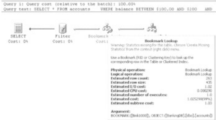
Figure 4.26: Graphical query execution plan for query 3 showing the bookmark warning
