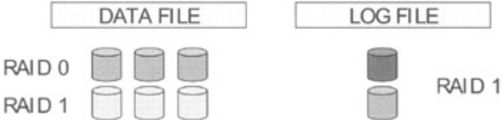
Figure 5.19: A RAID configuration utilizing RAID 0 and 1 for the data and RAID 1 for the log
