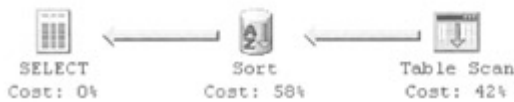
Figure 4.51: Graphical query execution plan showing an ORDER BY using a table scan rather than a nonclustered index
