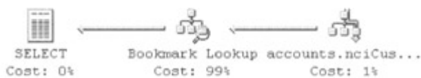
Figure 4.52: Graphical query execution plan showing an ORDER BY using a nonclustered index
