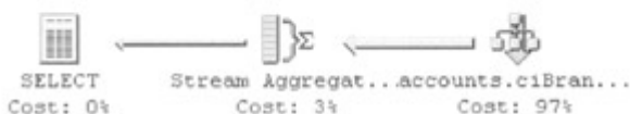
Figure 4.43: Graphical query execution plan showing a group by using a clustered index
