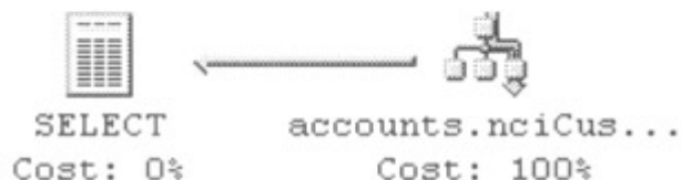
Figure 4.56: Graphical query execution plan showing an ORDER BY using a composite nonclustered index and a descending index key
