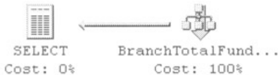
Figure 4.61: Graphical query execution plan for a query on a table with an indexed view
