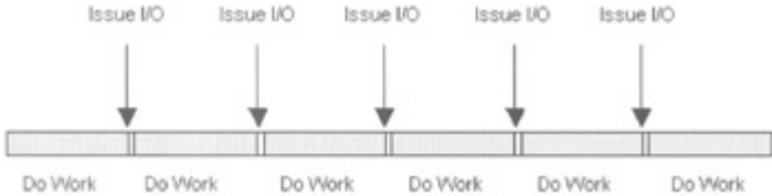
Figure 5.24: Performing a table scan with read ahead
