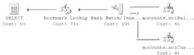
Figure 4.28: Graphical query execution plan for query 3 with two nonclustered indexes
