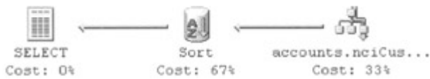
Figure 4.55: Graphical query execution plan showing an ORDER BY using a composite nonclustered index and a descending order
