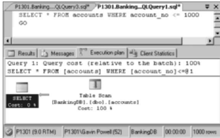
Figure 8.14 Increase row count and index + table scan becomes full table scan
