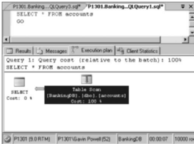
Figure 8.10 A non-clustered primary key forces a full table scan
