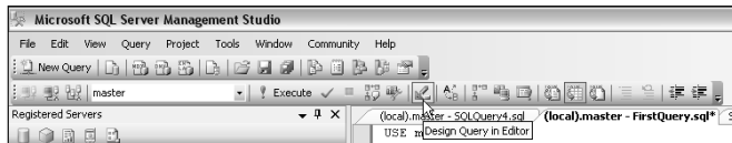
Figure 3-8: The SQL Editor toolbar and the button to open the Query Designer.
