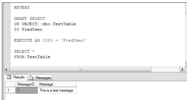
Figure 18-1: Successful execution of a SELECT statement after the SELECT permission is granted.
