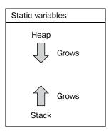
The stack grows toward the heap when a method is invoked and shrinks when the method returns. The heap does not grow in a predictable order and can become fragmented. As they share the same memory space, if the heap and stack collide then the program will terminate.
