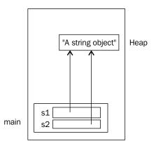
The new keyword was used in this situation to ensure that the string object is allocated from the heap. If we had used a string literal, as shown below, the object is allocated to an internal pool as discussed in the *String comparisons* section in *Chapter 2, Java Data Types and Their Usage*:
