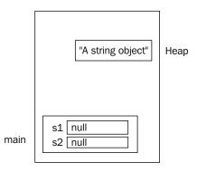
There exists a JVM background thread, which executes periodically to reclaim the unused objects. At some point in the future, the thread will execute. When an object is ready to be reclaimed, the thread will do the following:
