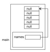
When a string is assigned to an element of the array, the array element is modified to reference that string as illustrated as follows:
