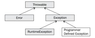
There are numerous pre-defined errors that are derived from the Error and RuntimeException classes. There is little that a programmer will do with the exceptions derived from the Error object. These exceptions represent problems with the JVM and normally can't be recovered. The Exception class is different. The two classes that derive from the Exception class support two types of exceptions:
