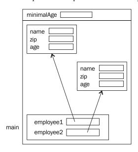
There is only one copy of each method for a class regardless of whether the method is an instance method or a static method. A static method is declared the same way as an instance method, except that the static keyword precedes the declaration of the method. The static setMinimumAge method, in the following code snippet, illustrates the declaration of a static method:
