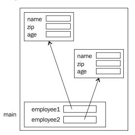
When a new object is created, a constructor for that object is executed. The purpose of a constructor is to initialize an object. This process is covered in the *Constructors* section. The class' methods are shared among the instances of the class. That is, there is only one copy of the methods.
