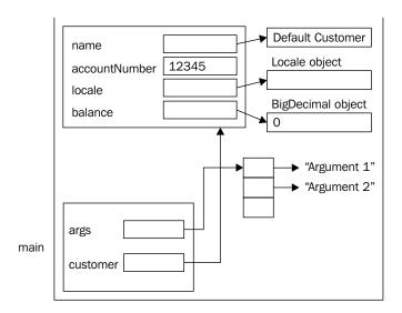
When the setBalance method is executed, its activation record is pushed onto the program stack as illustrated below. The setBalance method has a single parameter, balance, which is assigned to the balance instance variable. But first, it is used as an argument to the BigDecimal constructor. The this keyword references the current object.
