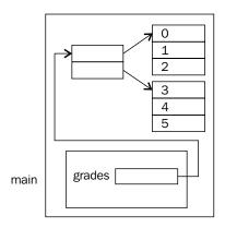
In a two-dimensional array, the rows do not necessarily have to be the same size. In the following code sequence, we create an array with different row lengths. Arrays of this type are called **ragged arrays**.
