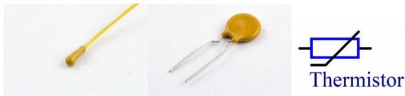
Figure 15 - Thermistor and its symbol
