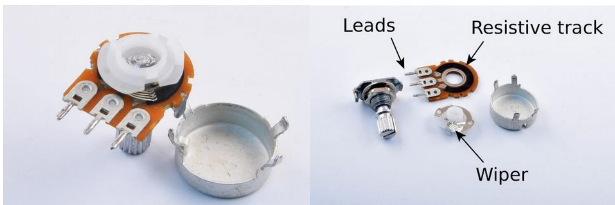
Figure 19 - Internal structure of potentiometer
