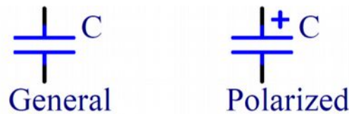
Figure 21 – Symbols of capacitors (unipolar and polarized)
