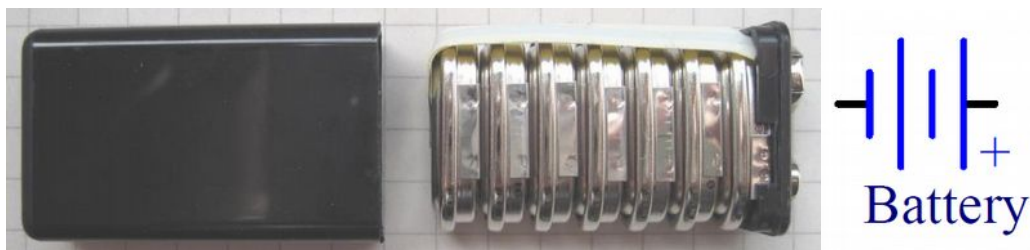
Figure 7 – Battery and its symbol
