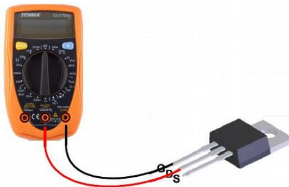
Figure 41 - Examination of gate-drain short circuit, in case of N-channel MOSFET
