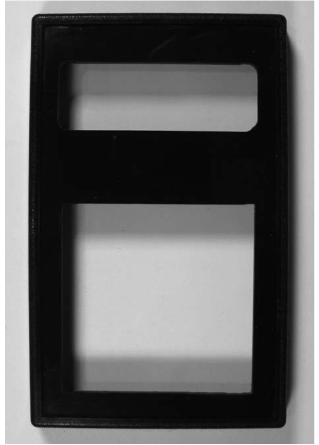
Figure 14-10 Top of the enclosure with the completed openings for the keypad and LCD
