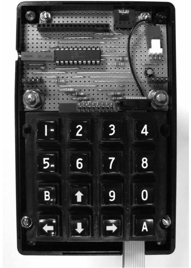
Figure 14-7 MPD with ribbon cable and keypad attached
