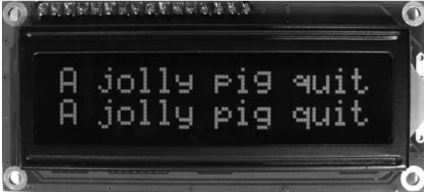
Figure 10-6 Comparison of LCD standard and custom characters
