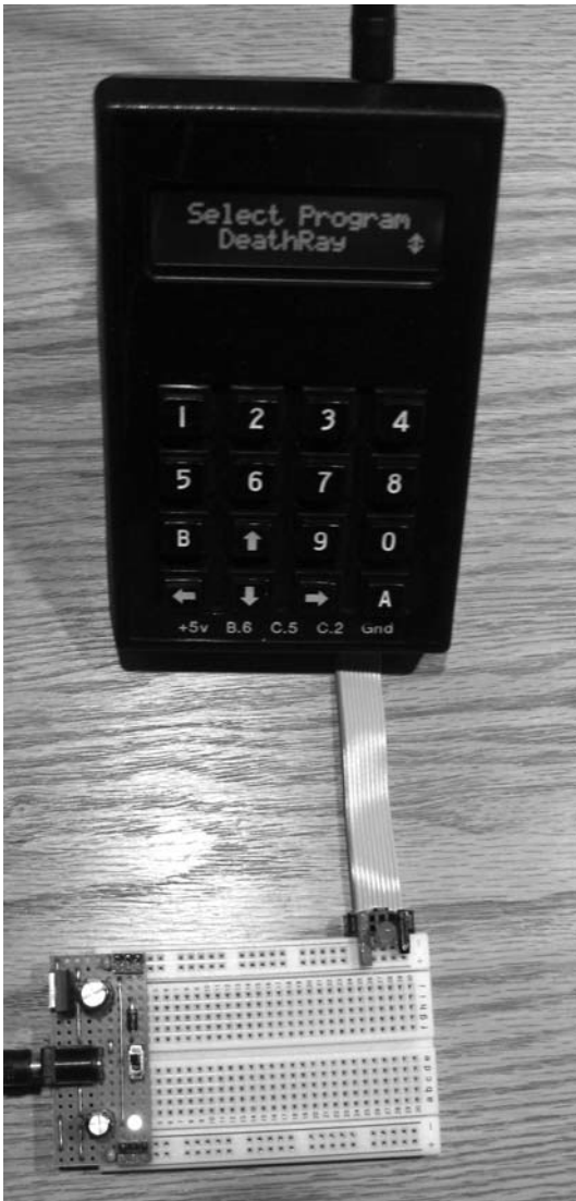
Figure 15-3 Breadboard circuit for testing the comparator 1 configuration
