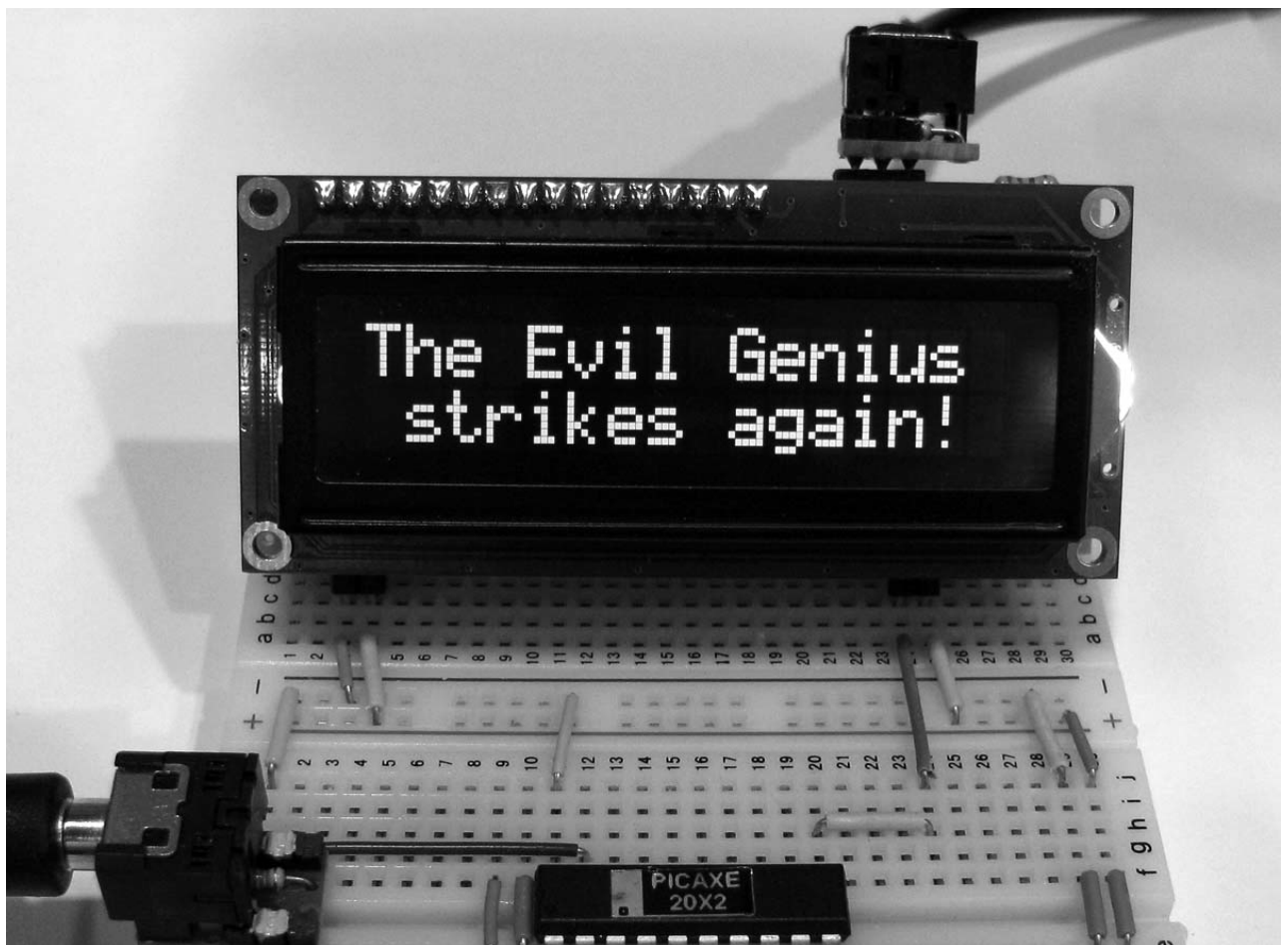
Figure 10-5 Breadboard setup for completed serial LCD project
