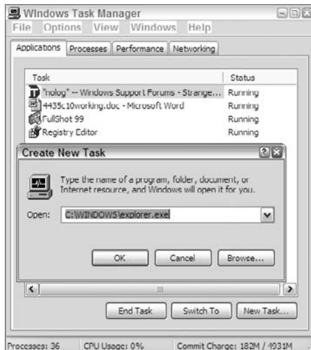
FIGURE 10.26 Using Task Manager's Create New Task dialog box to restart Explorer
