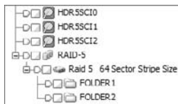
FIGURE 6.8 Three physical devices from a hardware RAID 5 configured and mounted as a logical RAID 5 within EnCase
