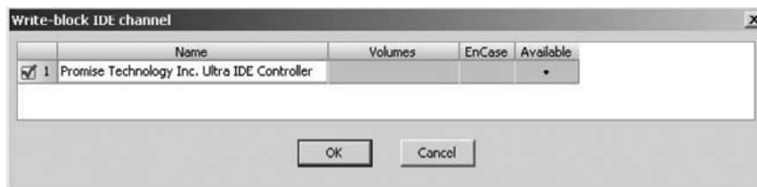
FIGURE 4.28 Select the channel to write-block in the Write-Block IDE Channel dialog box.
