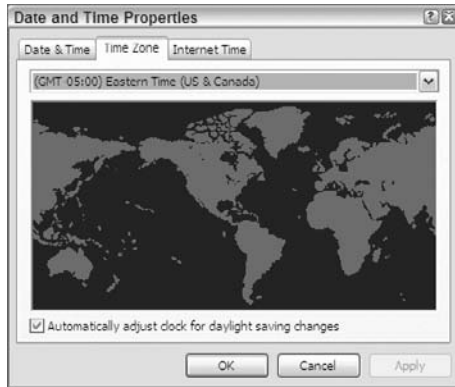
FIGURE 9.1 Windows Date and Time Properties dialog box showing the Time Zone tab on which the user sets the local time zone
