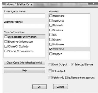
FIGURE 9.6 The Windows Initialize Case dialog box lets you extract and summarize time zone information in a bookmark.
