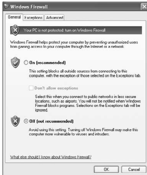
FIGURE 4.11 Windows Firewall options. Make sure Off is selected, or go to the Exceptions tab and add ENCASE.EXE as a program.
