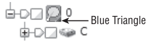
FIGURE 6.6 A live physical device and its associated volume. Note the icon for the physical device has a blue triangle in the lower right, indicating it is a live device.
