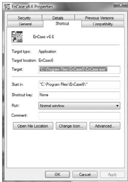
FIGURE 9.26 Shortcut tab of the Properties dialog box for a shortcut or link file
