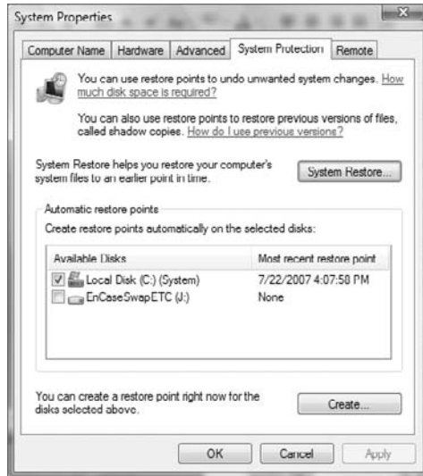
FIGURE 9.56 System Protection tab of Windows Vista System Properties menu
