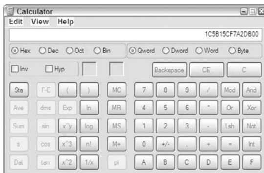
FIGURE 9.5 The Windows 64-bit time stamp is entered in a scientific calculator in reverse order because it is stored in little endian format.
