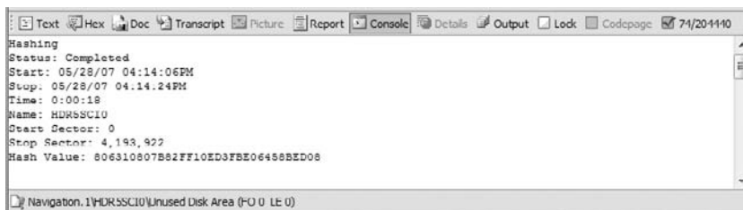
FIGURE 6.34 The Console view after receiving data from a completed hashing routine
