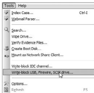
FIGURE 4.30 The Write-Block USB, Firewire, SCSI Drive option on Tools menu
