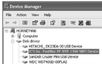
FIGURE 4.19 When FastBloc is successfully detected and mounted by Windows PnP, FastBloc is listed under Disk Drives, as shown here in Windows XP Device Manager.
