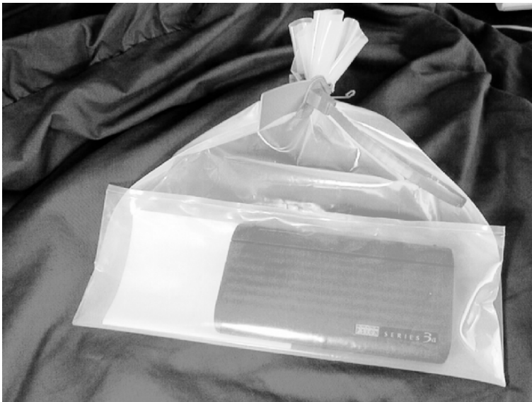
Fig. 8.8 How not to seal an organizer in an evidence bag (photograph: Tony Sammes and Brian Jenkinson).
