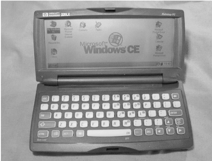
Fig. 8.2 A Windows CE organizer – the HP 320 LX (photograph: Tony Sammes and Brian Jenkinson).
