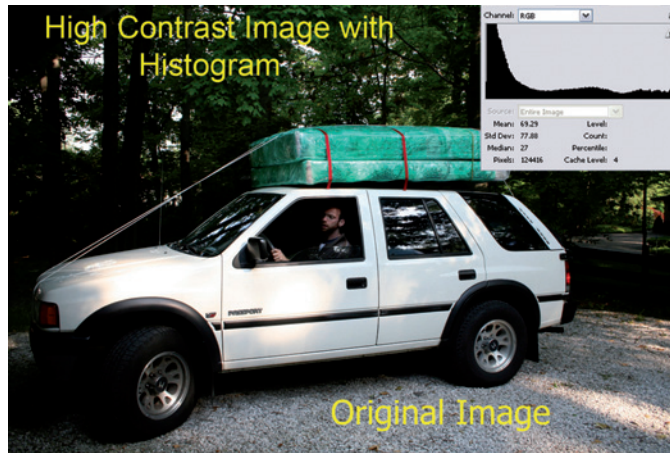
FIGURE 10.7 High Contrast Photo with Histogram. Shown are a contrasty photo and its associated histogram. Note that there are many pixels on the left and on the right and very few in the center.
