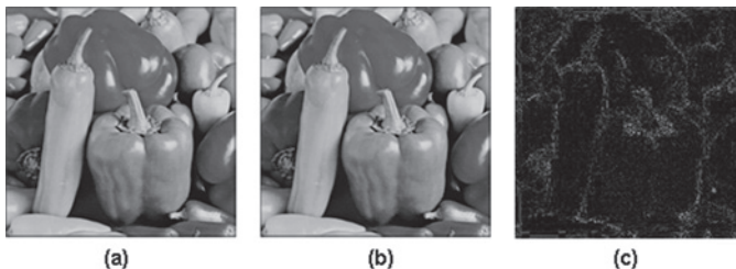
FIGURE 13.9 (a) Original image, (b) JPEG image, and (c) the difference between image (a) and (b).
