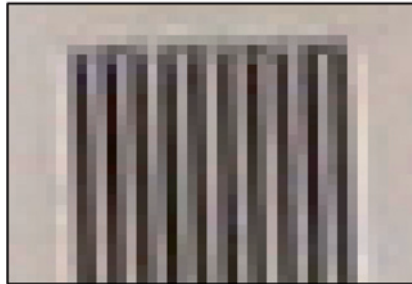
FIGURE 17.2 Digital Camera Image. Shown is a crop from a photo taken at just about the critical frame width. There were 10 bars on the chart and we can easily count the 10 bars in the image. The diagonal distortion was due to the fact that the bars and the pixel columns did not line up exactly.
