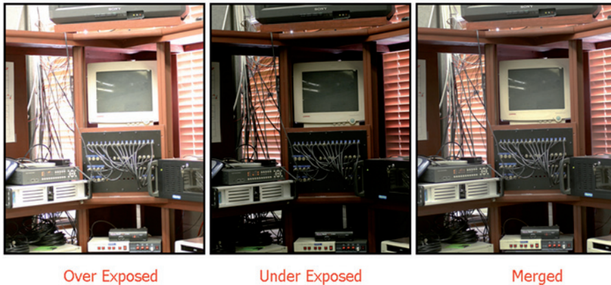
FIGURE 17.9 Extending Dynamic Range by Software. Five images of the same subject were taken at different exposure levels. The two extremes are shown on the left. These five were then merged using the High Dynamic Range tool in Adobe Photoshop software suite. The result is shown on the right.
