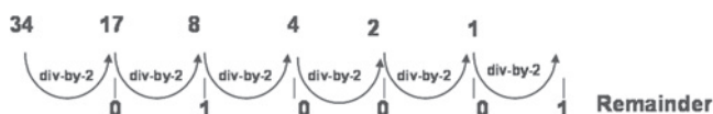
FIGURE 12.3 Illustrate a common practice of how to use divide-by-2 strategy for converting a decimal number 34_{10} to a binary bit pattern 100010_B .
