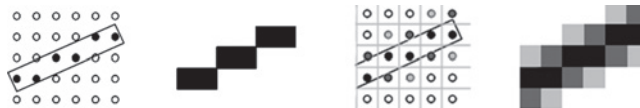
FIGURE 13.2 Image aliasing effect that results in jagged stairs-like patterns on the edge (left). Anti-aliasing can improve image aliasing problem (right).
