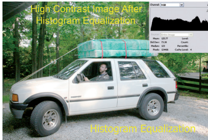
FIGURE 10.8 Effect of Histogram Equalization. This is the same image as shown in Figure 10.7, but after applying histogram equalization. The pixel values have been spread across the full brightness range.
