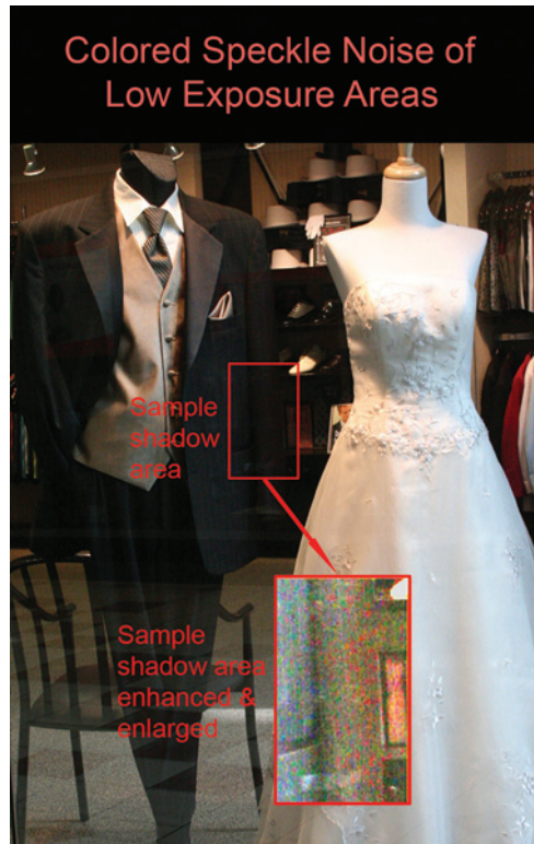
FIGURE 2.1 Colored Speckle Noise. In low exposure areas, digital photo sensors tend to exhibit random noise that is large compared to the low signal. In the figure, a dark portion of the image is brightened to show the speckle pattern inherent in that area.
