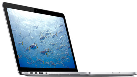
Physical screen sizes: 13.3" and 15.4" Resolutions: 2560x1600px and 2880x1800px PPIs: 227 and 220
