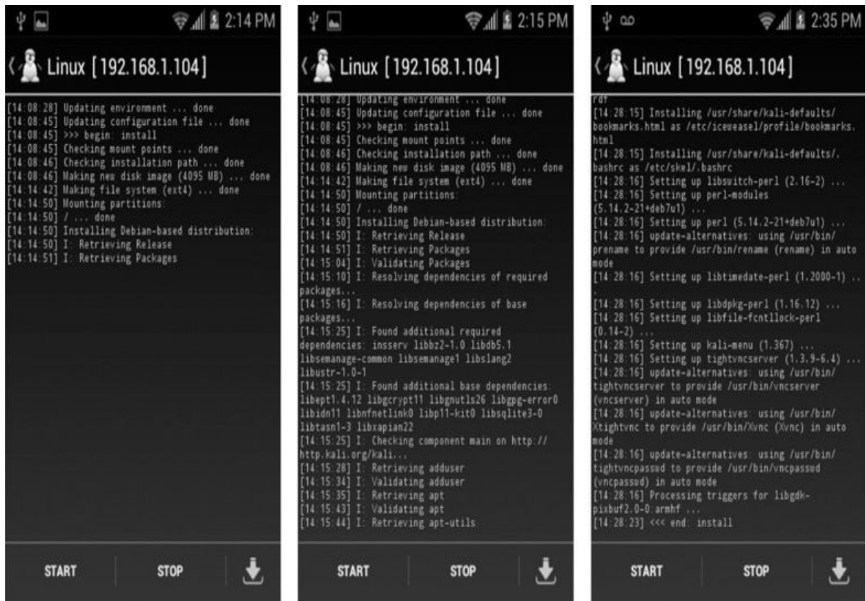
Figure 8-7 Initial Linux image installation messages
