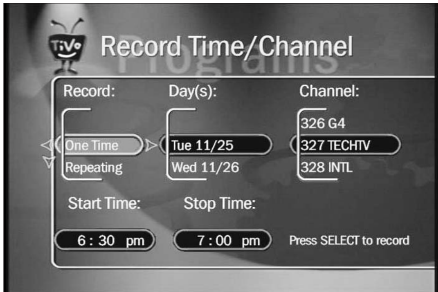
Figure 6-10: When necessary, TiVo can record a certain time slot on a certain channel, regardless of what’s playing.
