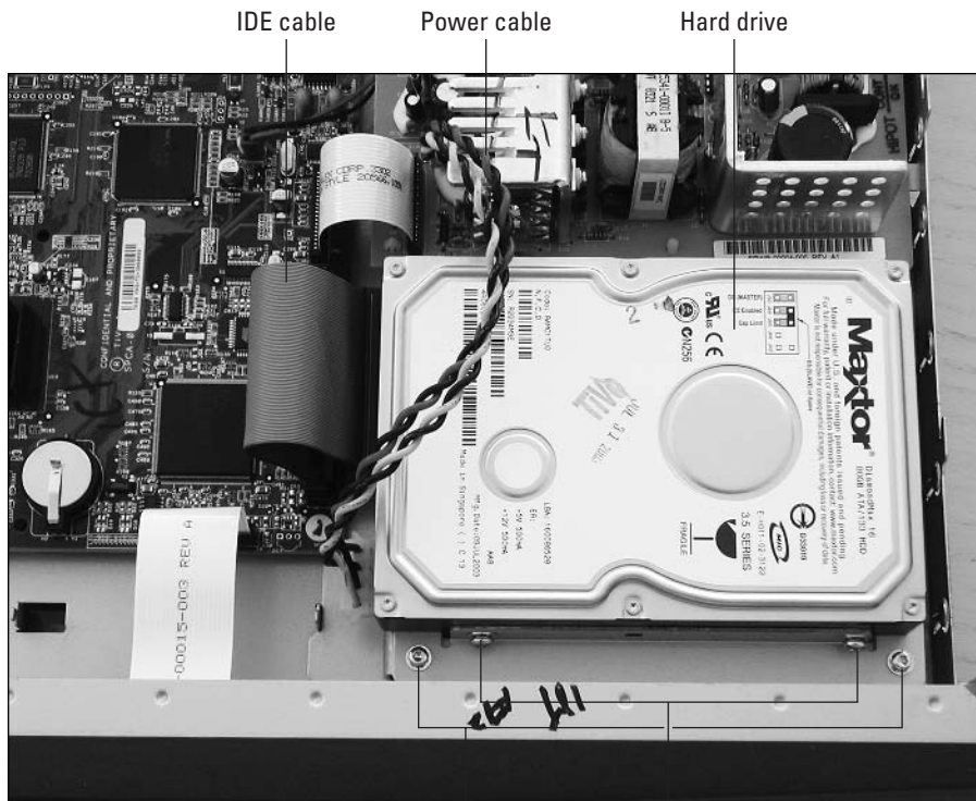
Screws holding drive to bracket
