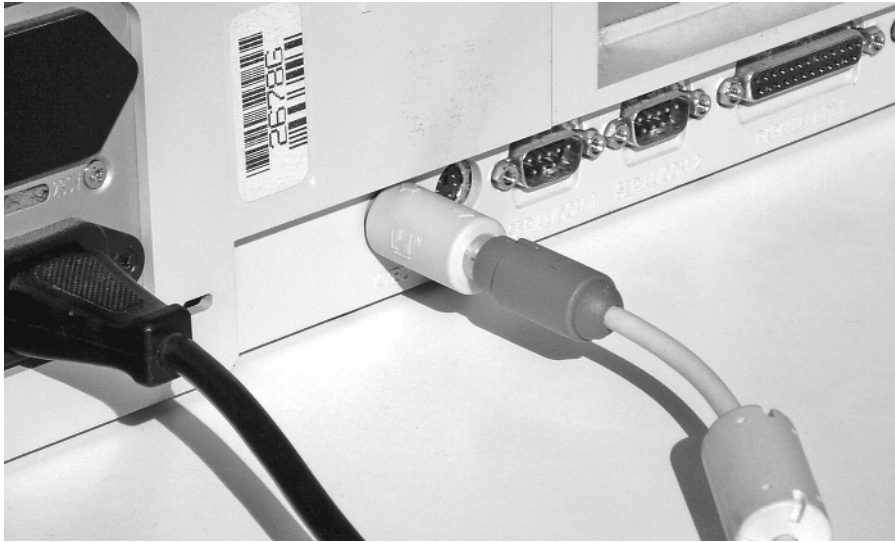
Figure 4-2 Keylogger device installed. Courtesy of Allen Concepts, Inc. ( www.keycatcher.com ).
