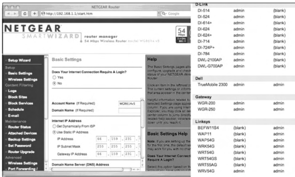
Figure 4.8 Netgear DSL Router Web Interface
