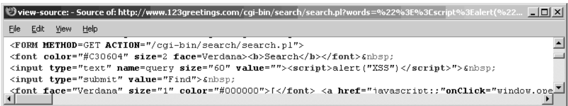
Figure 3.33 View Source of the Necessary XSS Payload
