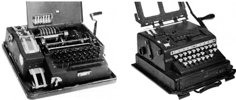
Fig. 73. Left: BC-543 (Hagelin Cryptograph Company, USA) Right: German copy Schlüsselgerät 41 (SG 41, Hagelin: C-41) by Wanderer Werke
