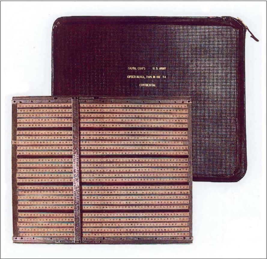
Strip cipher M-138-T4 used by the U.S. Army and U.S. Navy in the Second World War, based on a proposal by Parker Hitt in 1914. The 25 removable paper strips were numbered and used in prearranged order. The encryption was cryptologically equivalent to the M-94.
