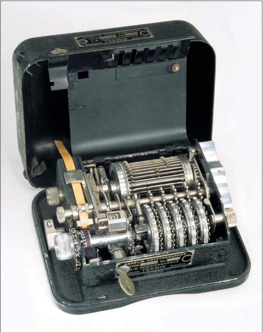
The Hagelin cipher machine 'Cryptographer' C-36, made by the Aktiebolaget Cryptoteknik, Stockholm, in 1936, has self-reciprocal encryption by BEAUFORT encryption steps performed by the 'lug cage', an invention of Boris Hagelin. The irregular movement is based on the use of keying wheels with different graduation, namely with 17, 19, 21, 23, and 25 teeth, which gives a key period of length 3 900 225. For such a purely mechanical machine, this was a pioneering achievement.
