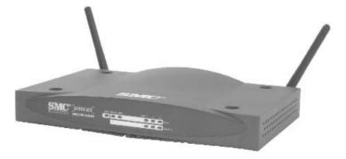
**Figure 8.17** The SMC Networks Barricade broadband router consists of an access point, a router and a three-port 10/100 Mbps Ethernet switch in a common housing.
