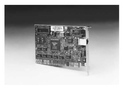
**Figure 3.43** The 3Com Corporation Fast Etherlink PT NIC supports the use of the EISA bus. (Photograph courtesy of 3Com Corporation.)
