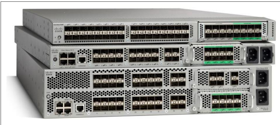
Figure 18-3. Nexus 5500, 5010 and 5020; courtesy of Cisco Systems, Inc.; unauthorized use not permitted
