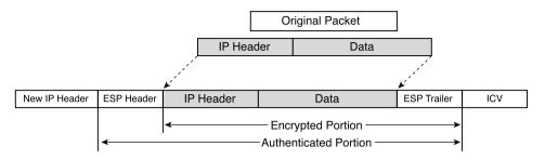
ESP supports NAT in either Tunnel or Transport mode, and only ESP supports encryption. If you need encryption, you must use ESP. If you also want authentication with ESP, you must select ESP HMAC service. HMAC uses the MD5 and SHA-1 keyed hashing algorithms.
