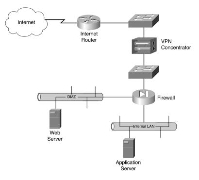
Figure 3-4 shows the VPN concentrator placed behind the firewall.
