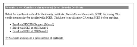
Enroll via SCEP. . . options are only available on this screen if you installed the CA certificate using SCEP. In this case, two CA certificates were installed using SCEP.
