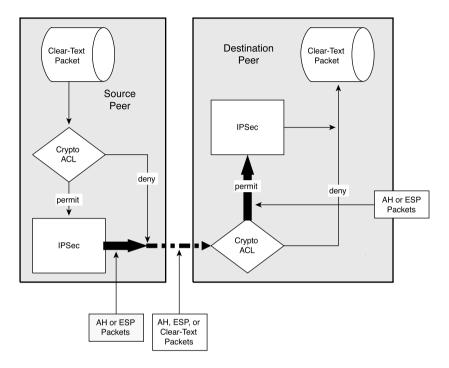
When these **permit** and **deny** keywords are used in the proper combinations, data are successfully protected and transferred. When they are not used in the proper combinations, data are discarded. Table 2-10 shows the various **permit** and **deny** keyword combinations and the actions that result from the combinations.
