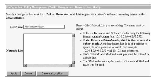
Network lists must be reflexive on opposite sides of the VPN connection. The networks listed as being "inside" on one concentrator should reflect those listed as "outside" on the other concentrator. Should a specific network be unreachable through a VPN connection, one of the first items to check is that the network lists on both sides show the "missing" network.
