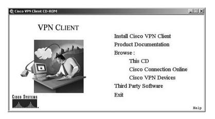
Click the option to **Install Cisco VPN Client**. The system might respond with a message like the one shown in Figure 4-28, stating that the installer needs to disable the IPSec Policy Agent. Simply click the **Yes** button to continue the installation process.
