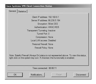
This screen shows the client IP address and the server IP address. Next, you see the encryption and authentication used for this connection. Then, you see whether transparent tunneling is active. If it is, the tunneling port number is shown. This is followed by the compression in use and a notation regarding the local LAN access. If a personal firewall were in effect, it would be listed here. Any firewall policy in use, such as AYT or CPP, is shown.
