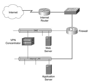
Figure 3-6 shows the VPN concentrator placed in the firewall's DMZ.
