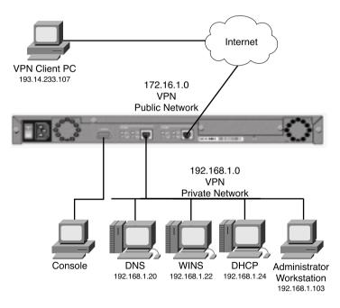
You need to attach a console for the initial configuration. The console port takes a standard straight-through RS-232 serial cable with a female DB-9 connector, which Cisco supplies with the system. Once the Private interface has been configured, you can access the concentrator from your administrator workstation using a web browser such as Internet Explorer or Netscape Navigator.
