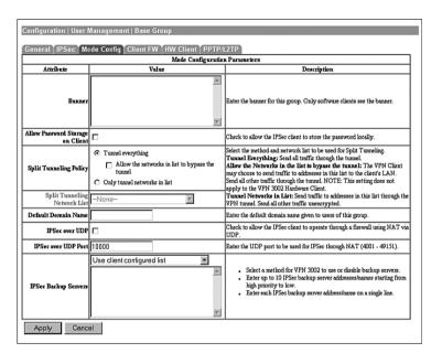
Figure 9-9 Configuration | User Management | Base Group | Mode Config
