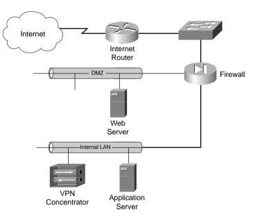
Figure 3-5 shows the VPN concentrator placed parallel with the firewall.
