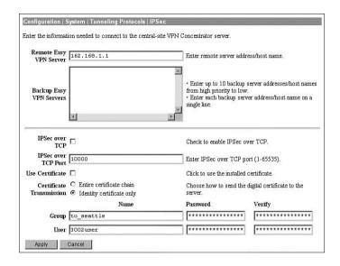
Figure 8-3 Configuration | System | Tunneling Protocols | IPSec
