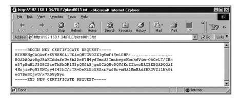
With the PEM version of the certificate request in hand, you now contact your CA operator and transmit the request. You could do that via HTTP, FTP, or e-mail, or by copying the request to a portable medium and physically transporting the request to the CA operator. Once the CA operator has accepted your request and enrolled it in the CA system, the CA operator returns
