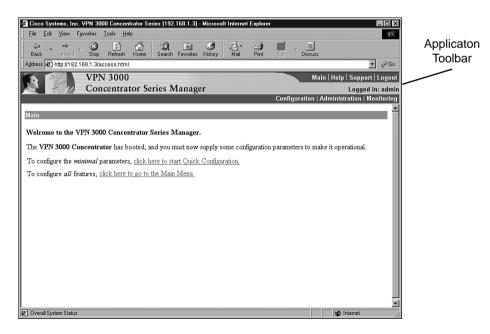
The top portion of the screen is the application toolbar, and it is displayed on every other manager screen. Because this is a consistent header, it is not shown in subsequent screen displays.
