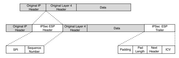
Figure 2-7 shows more detail about the lengths and placement of the various ESP components.
