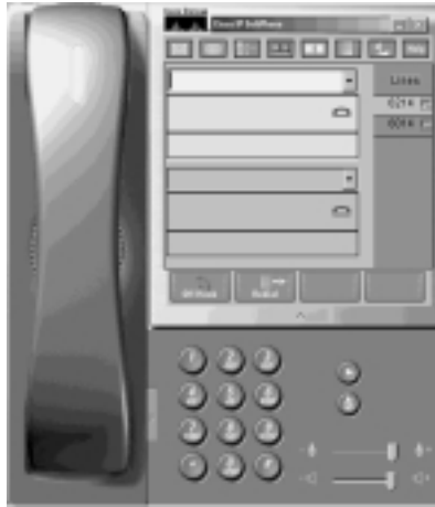
Figure 10.16 The IP Soft Phone, a Replica of the Model 7960 Desktop Model
