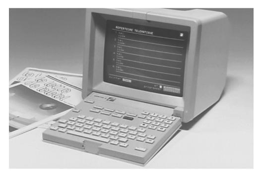
Figure 1.9 France Télécom's first minitel terminal (1981) [reproduced courtesy of France Télécom].
