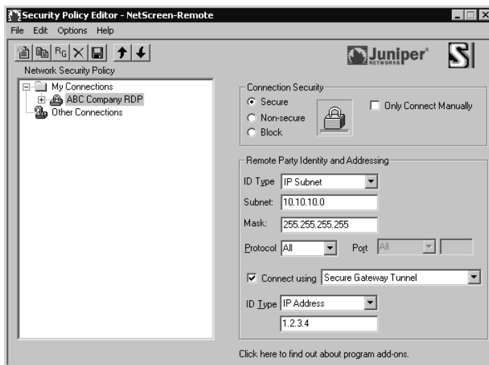
Figure 11.13 Initial Configuration of NetScreen Remote
