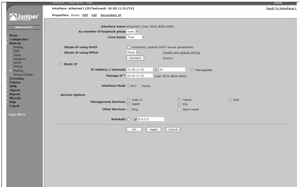
Figure 8.5 Web UI Screen Shot of Interface-Based Source NAT
