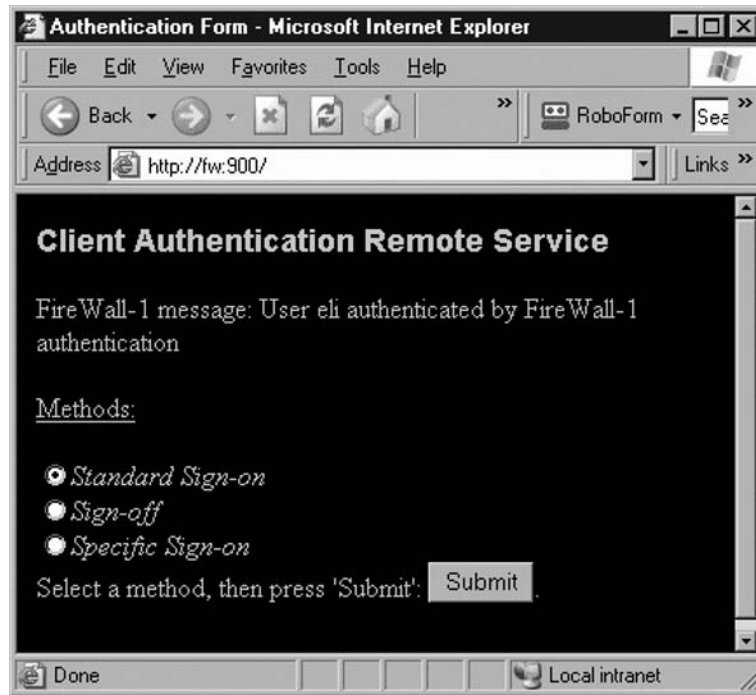
Figure 6.43 HTTP Manual Client Authentication—Selecting the Sign-In
