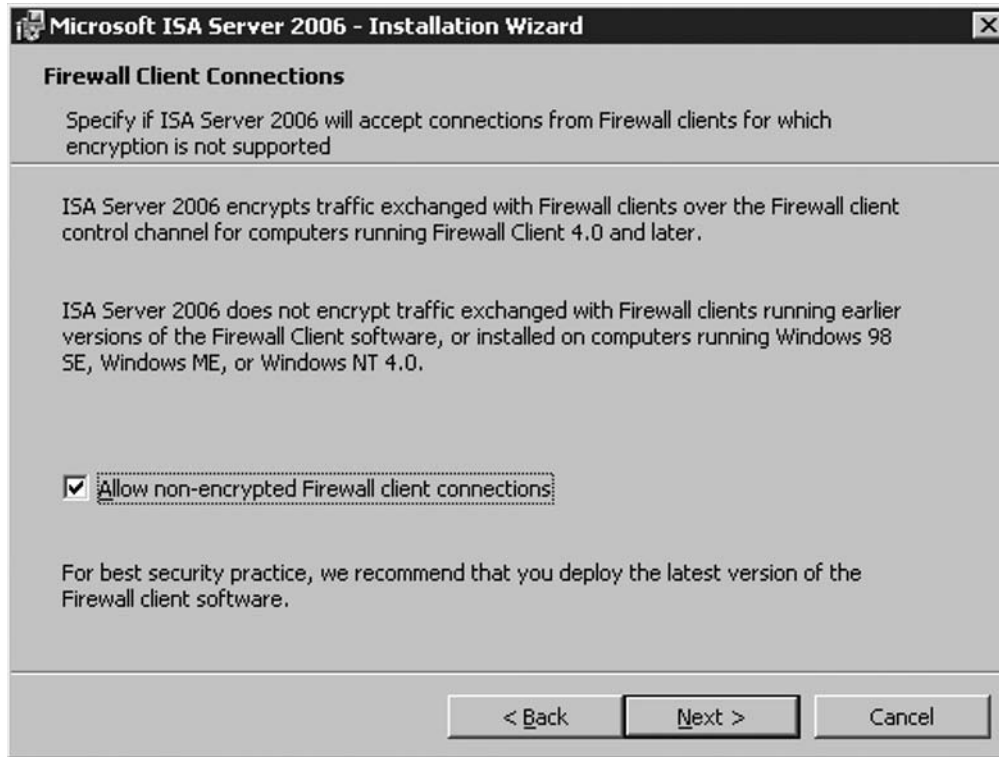
Figure 18.10 The Firewall Client Connection Settings Page
