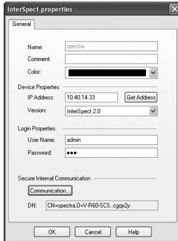
Figure 2.23 Check Point Interspect Object
