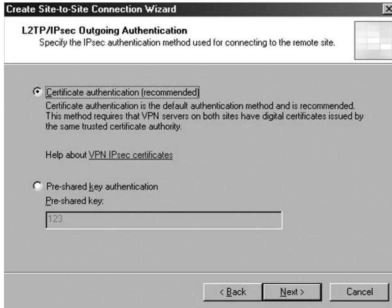
Figure 20.54 The Outgoing L2TP/IPSec Authentication method
