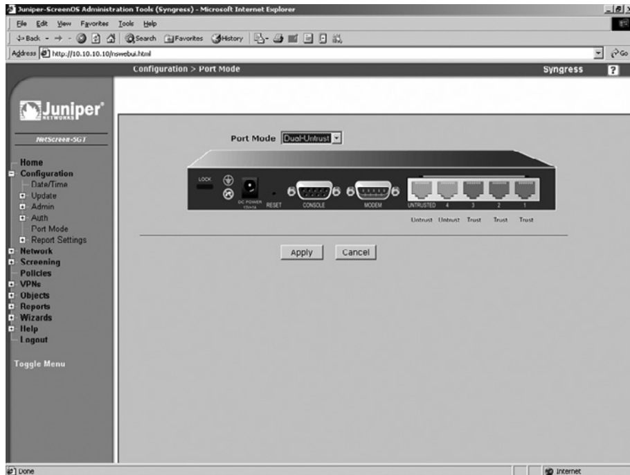
Figure 22.23 Port Mode Configuration
