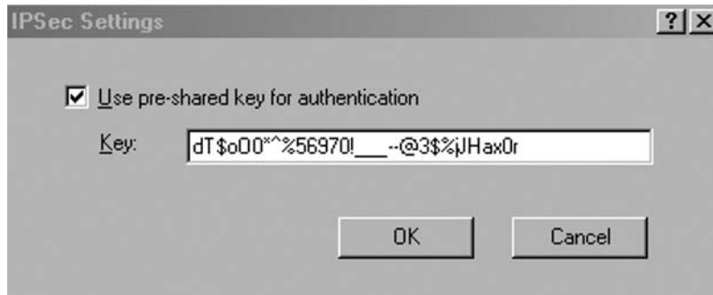
Figure 20.27 Enter a pre-shared key on the L2TP/IPSec client
