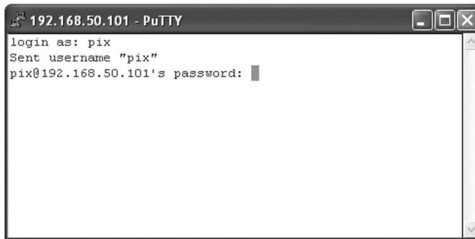
Figure 15.8 Using PuTTY and SSH to Login to a Cisco PIX
