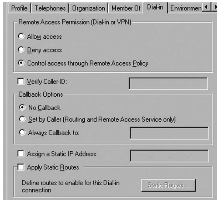
Figure 20.67 Controlling Access via Remote Access Policy
