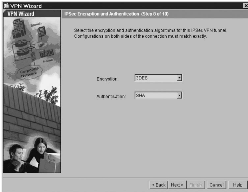
Figure 10.76 ASDM VPN Wizard IPsec Encryption and Authentication Screen
