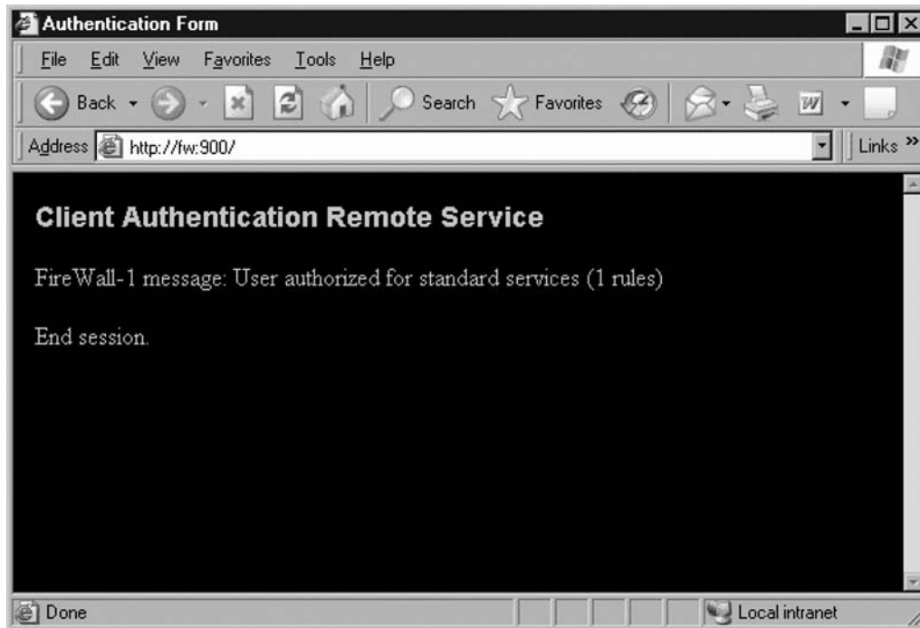
Figure 6.45 HTTP Manual Client Authentication—Successful Sign-In
