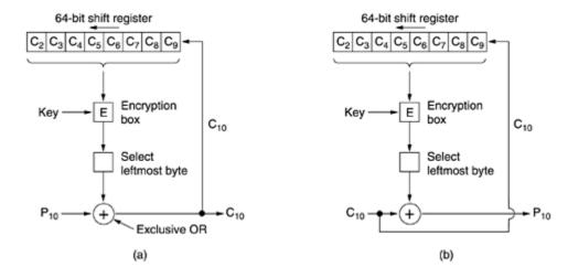
Decryption with cipher feedback mode just does the same thing as encryption. In particular, the content of the shift register is encrypted, not decrypted, so the selected byte that is XORed with C10 to get P10 is the same one that was XORed with P10 to generate C10 in the first place. As long as the two shift registers remain identical, decryption works correctly. It is illustrated in Fig. 8-13(b).
