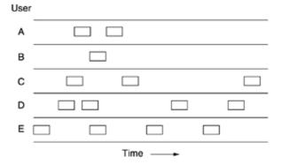
Whenever two frames try to occupy the channel at the same time, there will be a collision and both will be garbled. If the first bit of a new frame overlaps with just the last bit of a frame almost finished, both frames will be totally
