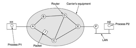
Figure 5-1. The environment of the network layer protocols.
