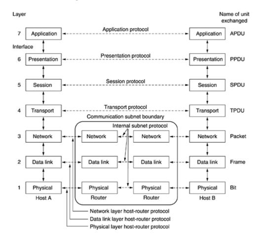
Figure 1-20. The OSI reference model.
