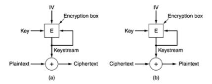
Decryption occurs by generating the same keystream at the receiving side. Since the keystream depends only on the IV and the key, it is not affected by transmission errors in the ciphertext. Thus, a 1-bit error in the transmitted ciphertext generates only a 1-bit error in the decrypted plaintext.
