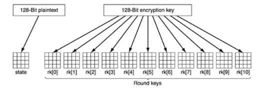
There is one more step before the main computation begins: rk[0] is XORed into state byte for byte. In other words each of the 16 bytes in state is replaced by the XOR of itself and the corresponding byte in rk[0].
