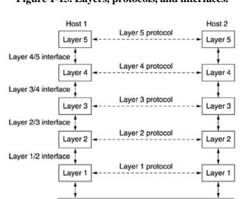
Figure 1-13. Layers, protocols, and interfaces.
