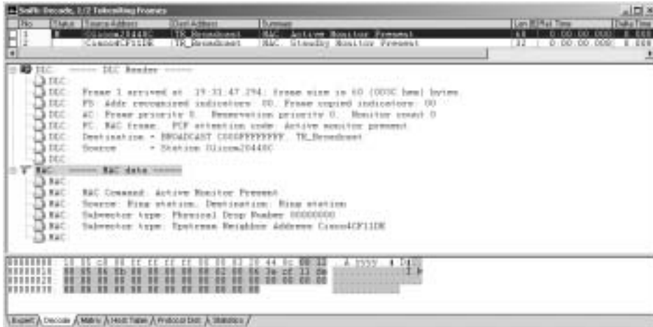
Figure 5.29 Viewing the Placement of Active and Standby Monitors
