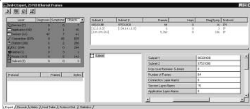
Figure 4.27 Viewing the Subnet Layer in the Expert to See IP and IPX Subnets
