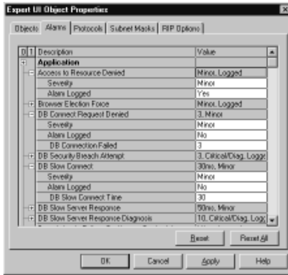
Figure 9.15 Expert Alarm Threshold Examples
