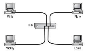
The design of a star topology resembles an old wagon wheel with the wooden spokes extending from the center point. The center point of the wagon wheel would be considered the hub. Like the wagon wheel, the network's most vulnerable point is the hub. If it fails, the whole system collapses. Fortunately, hub failures are extremely rare.
