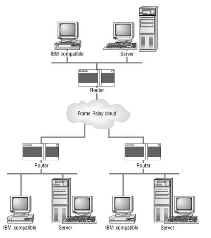
Frame relay uses permanent virtual circuits (PVCs). PVCs allow virtual data communications circuits between sender and receiver over a packet-switched network. This ensures that all data that enters a frame relay cloud at one side comes out at the other over a similar connection.
