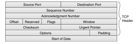
In addition to the source and destination port numbers, the sequence number, and the checksum, a TCP header contains the following information:
