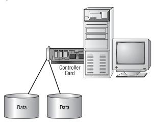
The drives do not need to be identical, but this helps. Both drives must have the same amount of free space to allow a mirror to be formed. For example, you have two 4GB drives; one has 3GB free, and the other has 2GB free. You can create one 2GB mirrored system.
