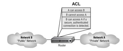
Note that data from users in Network A can pass through the router into Network B. IP spoofing attacks (in which someone, presumably a hacker, pretends to have a network address on the inside of a firewall to gain access to a network) can still occur if a user in Network B pretends to be located in Network A. (We'll discuss IP spoofing later in this chapter.)
