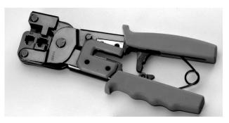
Many network technicians will make patch cables with a crimper. They will take a small piece of Category 5 UTP and crimp two RJ-45 ends on it to make the cable. Additionally, there are crimpers for the other types of cable, as well. There are even crimpers available for crimping on fiber-optic ends.
