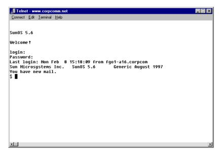
In today's Windows 95/98 and NT environments, Telnet is a basic GUI tool for testing TCP connections. You can telnet to any TCP port to see if it is responding, which is especially useful when checking SMTP and HTTP (web) ports. If you'll remember from Chapter 3, "TCP/IP Fundamentals," each upper-layer service in a TCP stack has a number for its address. Each network service that uses a particular address will respond to a TCP request
