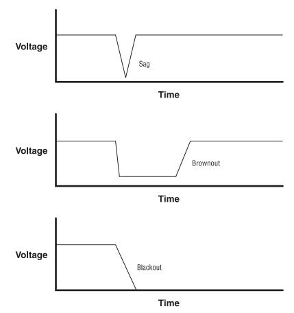
To ward off power underage problems, you need only one device: a UPS, which allows network devices to continue to function even in the complete absence of power. Some are intelligent and can shut down your computer in the case of a blackout.
