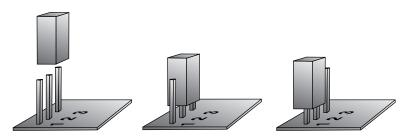
You'll often see devices with just three pins. These are common for devices that require only two settings, like on and off, or enabled and disabled.
