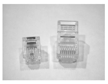
In almost every case, UTP uses RJ connectors. Even the now-extinct ARCnet used RJ connectors. You use a crimper to attach an RJ connector to a cable, just as you use a crimper with the BNC connector. The only difference is that the die that holds the connector is a different shape. Higherquality crimping tools have interchangeable dies for both types of cables.
