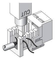
There are different blades and different types of punchdown tools. The most common is the punchdown with replaceable blades for the different types of connectors (either 66 or 110). Figure 6.22 shows an example of one of these types of punchdown tools.
