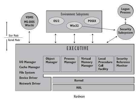
The two components to note in this diagram are the Hardware Abstraction Layer (HAL) and the many subsystems that can run applications. These two components enable NT to run many types of applications on many hardware types.
