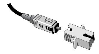
SC connectors work with either single-mode or multimode optical fibers, and they will last for around 1,000 matings. They are seeing increased use, but aren't as popular as ST connectors for LAN connections.
