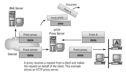
Proxies are good firewalls because the entire packet is dissected, and each section can be examined for invalid data at each layer of the OSI model. For example, a proxy can examine a packet for information contained in everything from the packet header to the contents of the message. Attachments can also be checked for viruses. Messages can be searched for keywords that might indicate the source of a packet.
