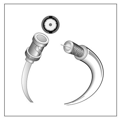
With Thinnet cable, you use *BNC* connectors (see Figure 1.15) to attach stations to the network. It is beyond my province to settle the long-standing argument over the meaning of the abbreviation BNC. BNC could mean BayoNet Connector, Bayonet Nut Connector, or British Navel Connector. What is relevant is that the BNC connector locks securely with a quarter-twist motion.
