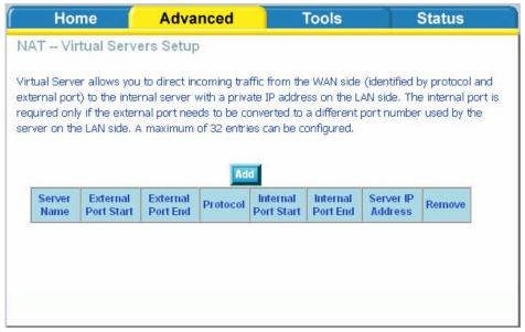
Select the virtual server from the drop-down list and complete the server IP address, then click on **Apply** once.
