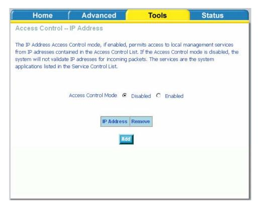
To assign the IP address of the management station that is permitted to access the local management services, enter the IP address in the box and click on the **Apply** button.
