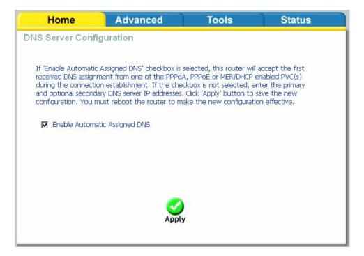
If you uncheck the *Enable Automatic Assigned DNS* checkbox, two additional fields—primary and secondary DNS server—will appear. Enter the information and click on **Apply** to save the configuration.
