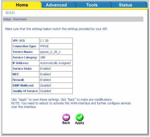
After you apply the configurations, it will return to the WAN Setup screen showing the new configurations. Select the **Finish** button to save the changes and reboot the router.
