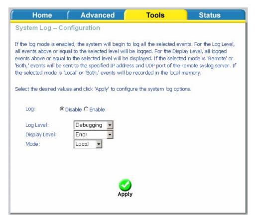
If the log is enabled, the system will log selected events including *Emergency*, *Alert*, *Critical*, *Error*, *Warning*, *Notice*, *Informational*, and *Debugging*. All events above or equal to the selected log level will be logged and displayed.
