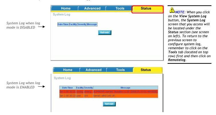
To configure the system log settings, click on the **Configure System Log** button to view the following screen.
