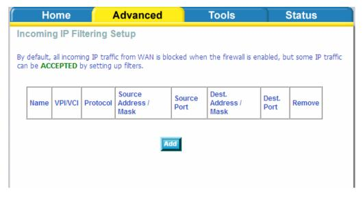
Enter a filter name, information about the source address (from the WAN side), and information about the destination address (to the LAN side). Select the protocol and WAN interface, then click on **Apply** to add the setting.
