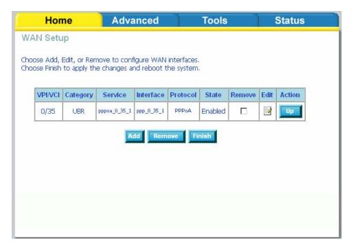
Click on the **Add** button if you want to add a new connection for the WAN interface and to proceed to the ATM PVC Configuration screen as seen below. The ATM PVC Configuration screen allows you to configure an ATM PVC identifier (VPI and VCI) and select a service category.
