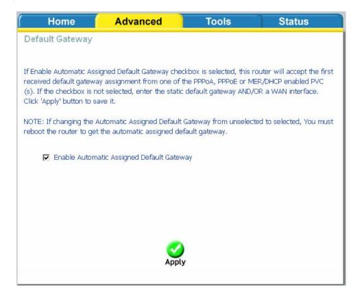
If you uncheck the **Enable Automatic Assigned Default Gateway** option, the below screen will be shown. Enter the default gateway IP address or select the established gateway to be used.
