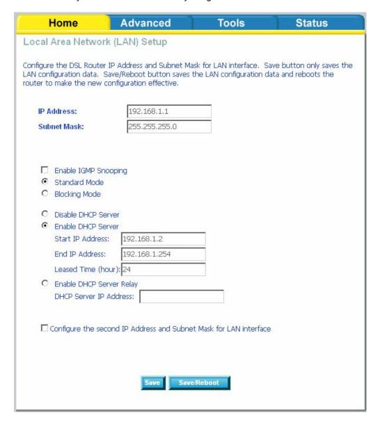
The **Save** button only saves the LAN configuration data, but does not apply the configurations. Select the **Save/Reboot** button to save the LAN configuration data and reboot the router and apply the new configurations.
