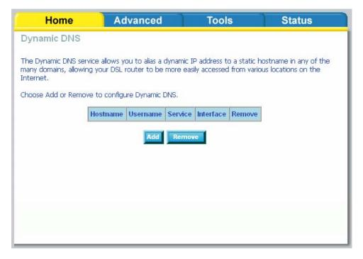
This screen allows you to add a dynamic DNS address from DynDNS.org or TZO. First select the D-DNS provider—DynDNS.org or TZO—from which you have obtained a dynamic DNS address. Enter the hostname and the interface that you are using. Also enter the username and password assigned by the DNS service. Click on Apply to save these configurations.
