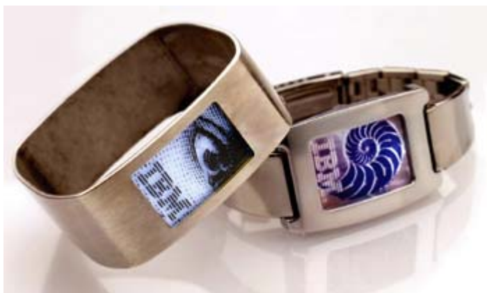
Figure 5.19: A prototype Bluetooth medic alert bracelet and watch, from IBM (Photo courtesy IBM Corporation)
