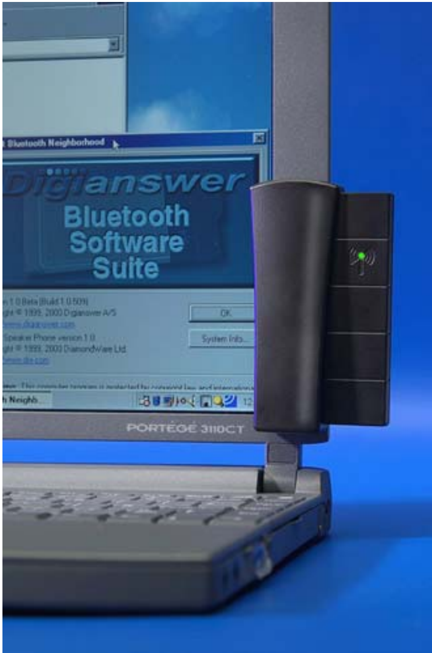
Figure 5.5: Digianswer's Bluetooth USB adapter, mounted on a notebook PC (Photo courtesy Digianswer A/S)
